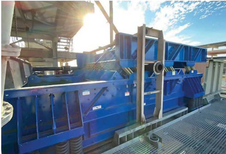
Sedibelo Resources’ Pilanesberg platinum mine in South Africa describes its 1.5-deck STM-SCREEN two-mass vibratory screen, above, as a game changer. (Photo: General Kinematics)
