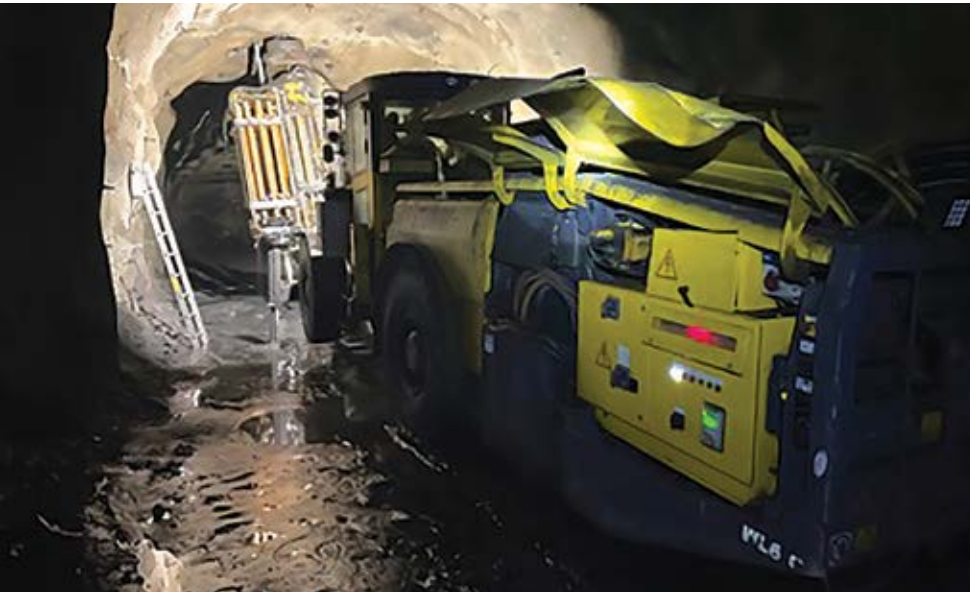
Four Simba E6 WLs, similar to the above, have each drilled 1 million meters at Malmberget mine. (Photo: Epiroc)
