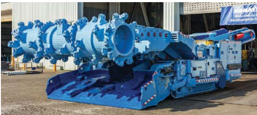
A blue Komatsu continuous miner arrives at the Mammoth mine site. (Photo: Coronado)
