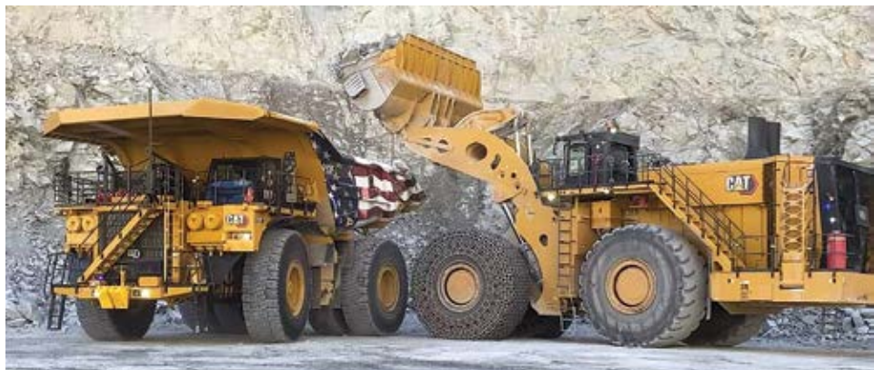
A wheel loader dumps ore into a haul truck at the Pinto Valley mine. (Photo: Capstone)
