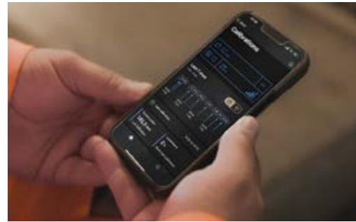
The ACS-s condition monitoring system for vibrating screens and feeders can be integrated with SAM, a cloud-based digital assistant, accessible by smartphone. (Photo: Sandvik)
