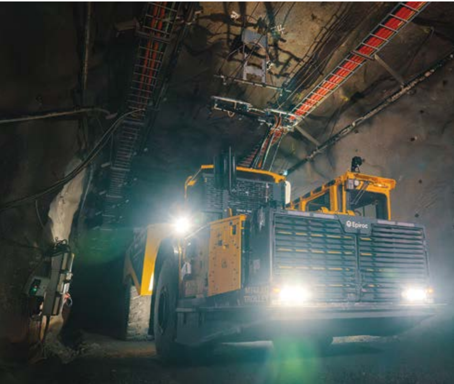
Trolley assist technology for underground haulage in use at Boliden's Ravliden operation in Sweden. (Photo: Epiroc, Boliden and ABB)
