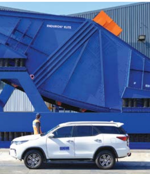
Above, the new ENDURON ELITE screen is designed for iron ore operations and for customers that prioritize high throughput. (Photo: Weir)
