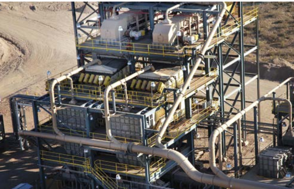
Above, MF Series banana screens are designed for high throughput with substantial undersize product in the feed. (Photo: Metso)
