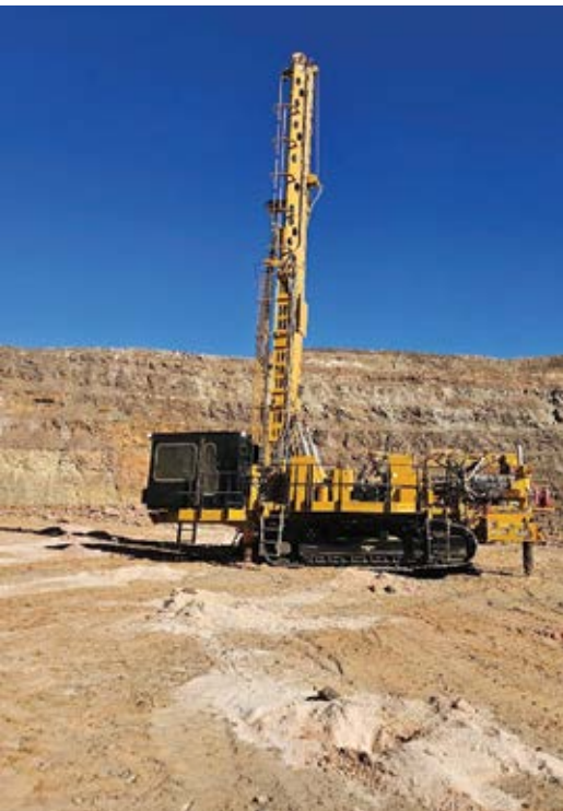
An ore control drill samples the Burro pit. (Photo: Gunnison)
