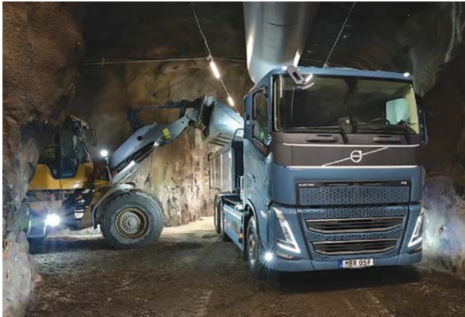
Boliden has used Volvo and Scania on-road trucks for underground hauling for many years and is now trialing battery electric versions of them. (Photo: Boliden)
